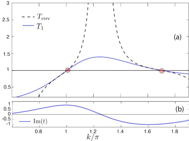
FIG. 2: Panel (a): The transmittance  $T_1$  (dashed) and the envelope function  $T_{\text{env}}$  (solid) around the  $\mathcal{PT}$ -broken parametric region where  $T_1 > 1$  for  $\gamma = 2.6$ . Panel (b): The imaginary part of the unit cell transmission coefficient  $t$  in the same region.
