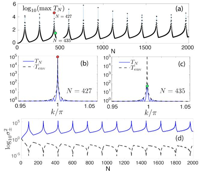
FIG. 4: Panel (a), (b) and (c): same as the corresponding panels of Fig. 3 but for the case of the electromagnetic slabs with parameters  $n_1 = 0.02$ , and  $\gamma = 1.1$ . Panel (d) shows the logarithm of the singular values  $\sigma_{\pm}^2$  of the scattering matrix as a function of the number of cells.
