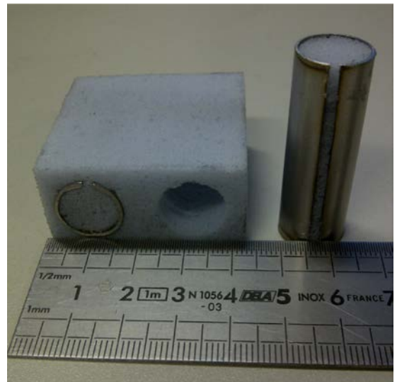
FIG. 8. (Color online) Picture of one of the characterized samples: “supercell” of two SRs with one of them taken out.
